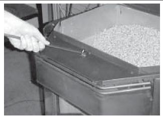
Figure 37 - Tube Scraper Rod
